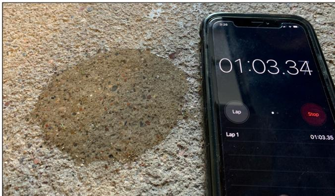
Figure 1. Water droplet partially absorbed after 1 minute indicating concrete is porous
